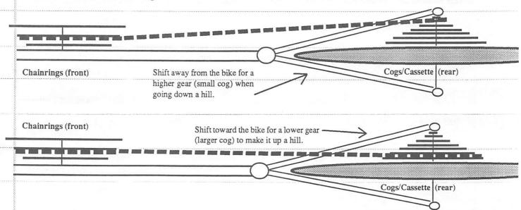
If the change in terrain is more pronounced, you will need to shift the front derailleur as well. And just to confuse you, the chain has the opposite effect here: Move it onto a smaller chainring (although still toward the bike) for a higher gear, and onto a larger chainring (away from the bike) for a lower gear.
